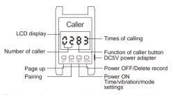
UP: in the standby status, press this button to browse the calling records from 0 to 9; in the pairing/deleting status, press this button to select number
